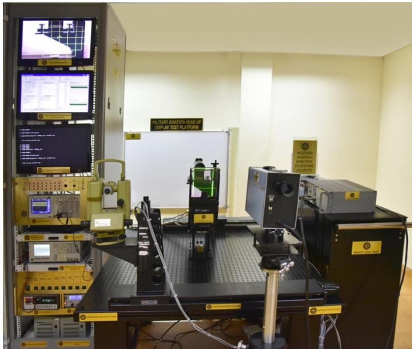
the process of automated testing & debugging less time consuming for Ground Staff and Maintenance Personnel using Intermediate Level (I-Level) & Operator Level (O Level) MAHTP at Defence Base Station, while system and subsystem level automated testing, fault rectification and maintenance is done using Depot Level MAHTP at Manufacturing Agency. The test platform provides following operations:
