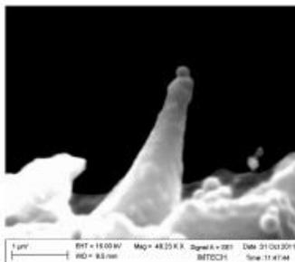
Antenna tweezed silica sphere as dipole antenna
