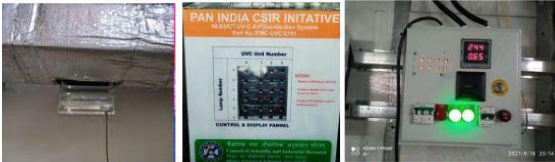
Fig.: Induct UVC disinfection system installed inside railway coach.
