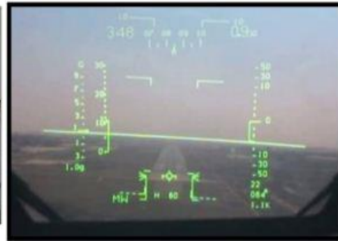
Flight Symbology viewed through HUD Mk1 in LCA-AF
