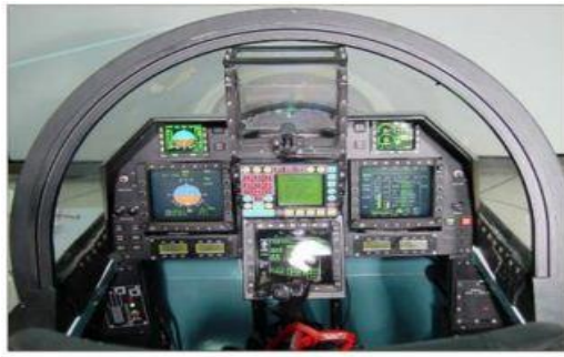
CSIO built Head UP Display Mk1 in LCA-AF Cockpit
