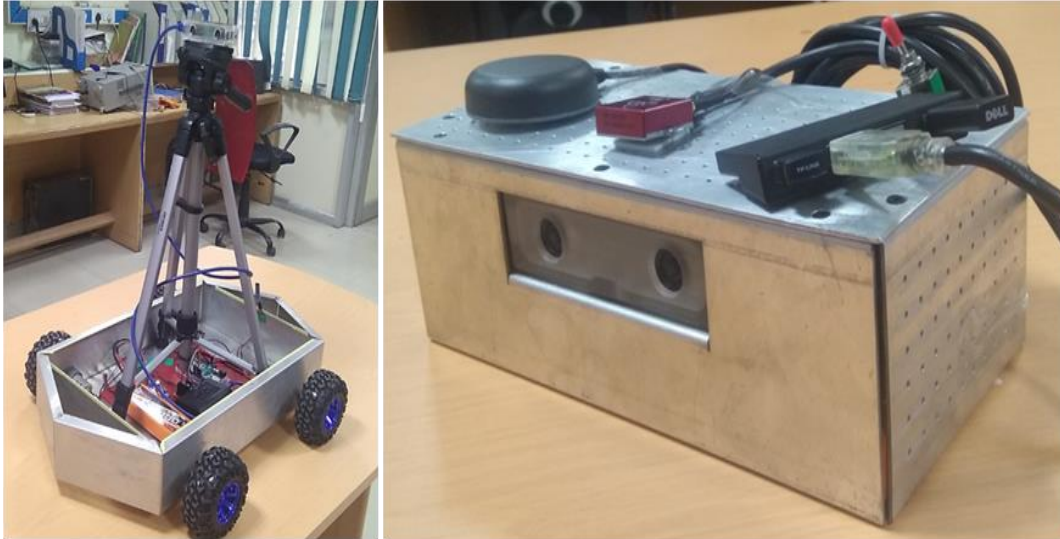
Dataset capturing in indoor environment using ground robot
