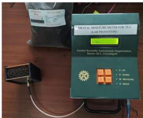
Lab Prototype: Hand held moisture Meter for Made Tea
