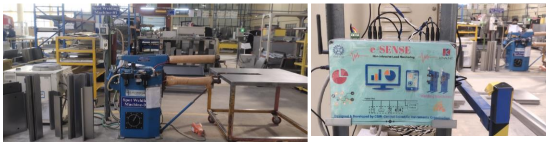
Typical view of deployment of e-SENSE in the industry for monitoring of five spot welding machine
