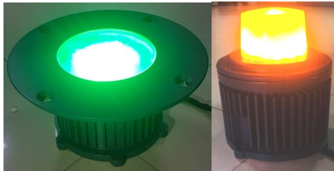
Functional Prototypes of two of the LRUs Visual Landing Aids
