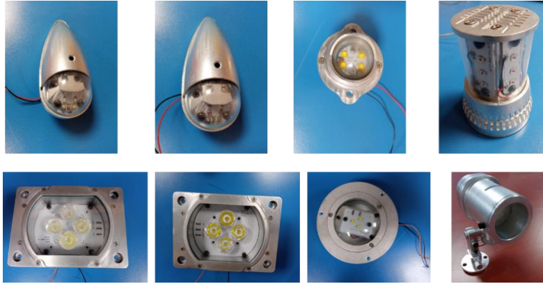
Form-Fit-Functional Units of LED Lights for HANSA-NG aircraft under testing at NAL Bengaluru
