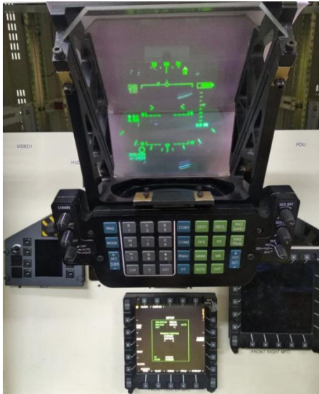
Rig & Aircraft Integration Testing of PDU
