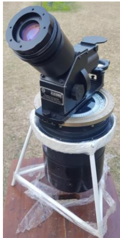
Marine Bearing Sight for Submarine integrated with the Bridge Bearing Repeater System
