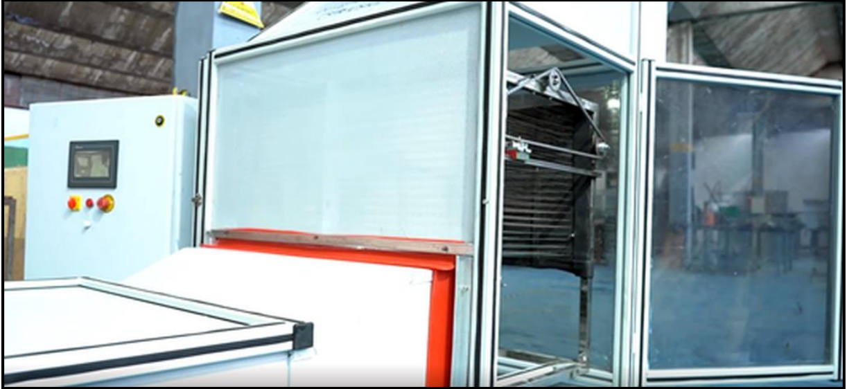
Nucleation Chamber, Instrumentation and Control System of the Snow Making Machine – designed and developed by CSIR-CSIO, Chandigarh
