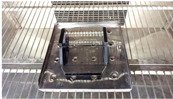
Glass Combiner assembly undergoing endurance test in Humidity Chamber
