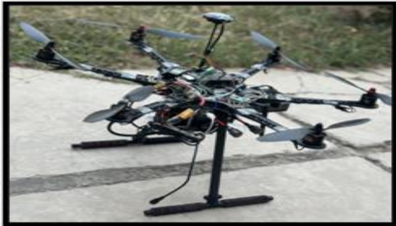
(Left): Customised UAV designed and developed at CSIR – CSIO for carrying out object detection and distance estimation on the UAV in real-time. (Right): Detected car in the image and its distance in meters
