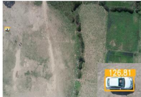
(Left): Customised UAV designed and developed at CSIR – CSIO for carrying out object detection and distance estimation on the UAV in real-time. (Right): Detected car in the image and its distance in meters
