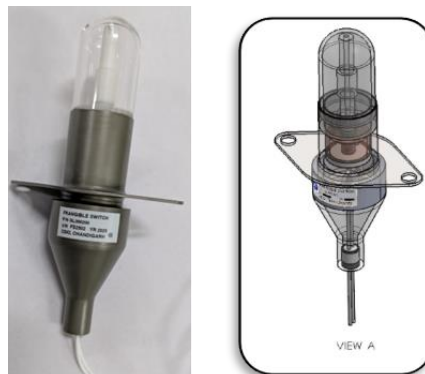
Developed prototype and schematic of aircraft crash detection switch
