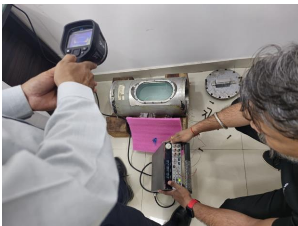
Head CAP Assembly of periscope during Heating testing
